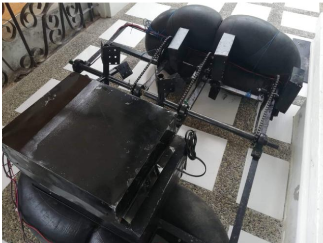
Fig. 7. The fuzzy logic controlled paddle wheel aerator.
