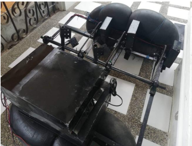
Fig. 7. The fuzzy logic controlled paddle wheel aerator.
