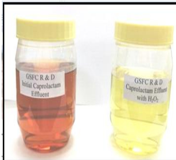
Fig. 9. Initial Caprolactam Effluent and after H 2 O 2 treatment
