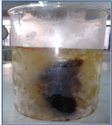
Fig. 5. Caprolactam effluent stream in frozen condition
