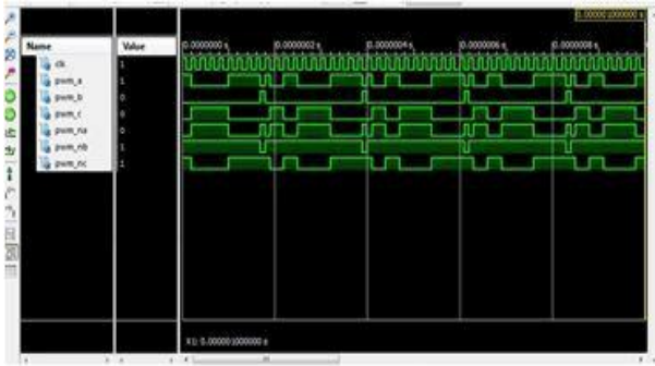
(6) Simulation of SVPWM module
