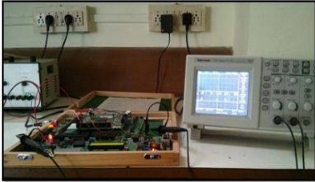
(7) PWM pulses observation on DSO
