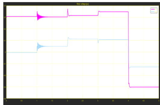
Figure.2. Rotor Output Voltage after Controller and Filter
