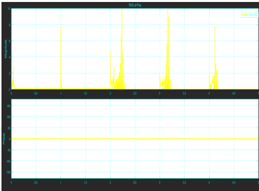
Figure.5. THD of Stator Power
