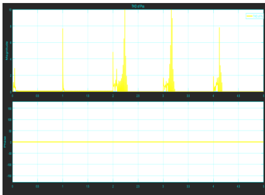
Figure.5. THD of Stator Power
