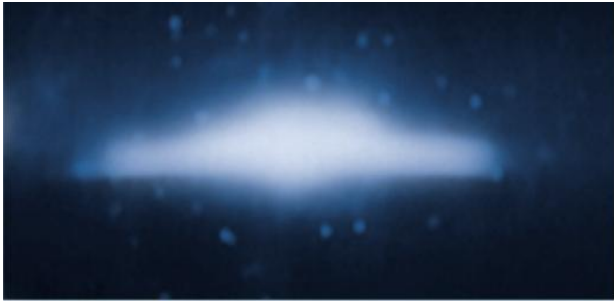
Fig. 4. Photograph of plasma discharge implemented in water.
