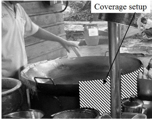
Fig. 1. Coverage setup (with texture) to reduce excess heat towards customer
