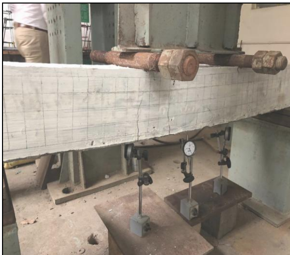
Fig. 5: Testing of RCC beams
