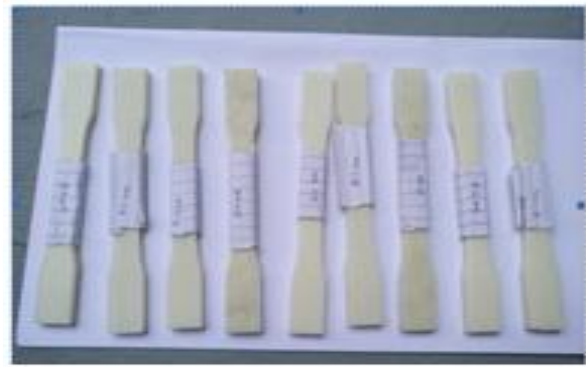
Fig. 2. 3D printed ABS specimens
