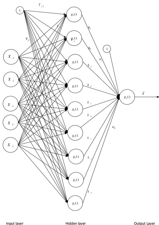
Figure 2.3. Multilayer perceptron neural network architecture model
