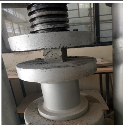
Figure 8 Failure mode of mortar cube
