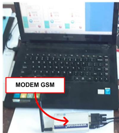
Fig. 5. The server is integrated with a GSM Modem
