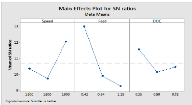
Fig. 4. Prediction of optimal set for better surface finish (Speed =1600 rpm, Depth of cut = 0.5 mm, Feed rate = 1.25 mm/rev)
