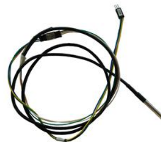
Figure 6. The water temperature sensor used in the study
