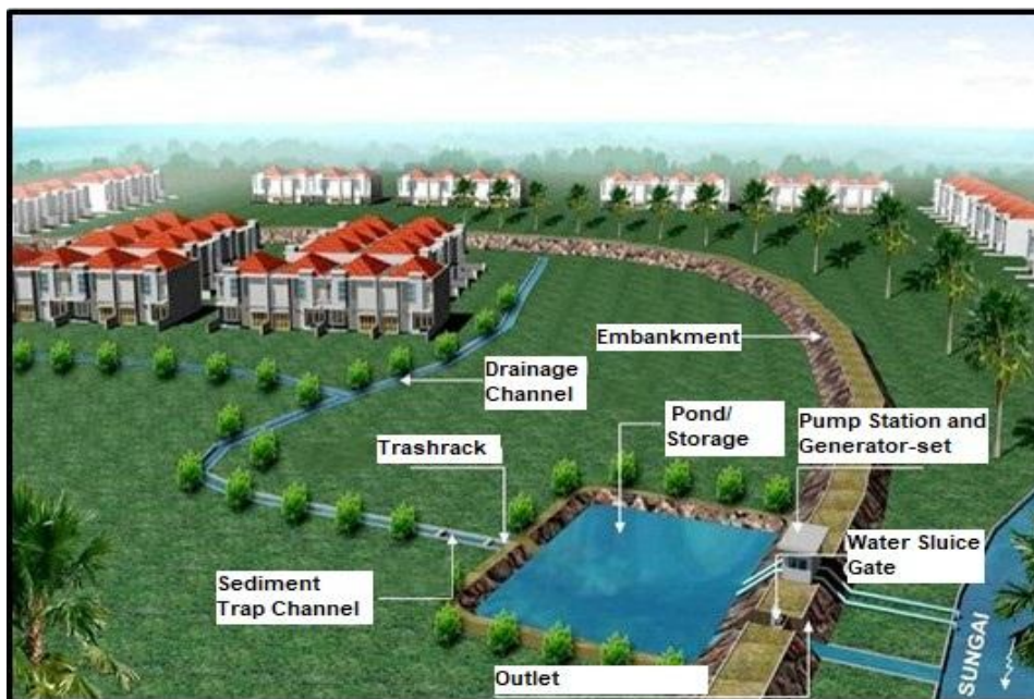
Fig. 1 Typical of Polder System
