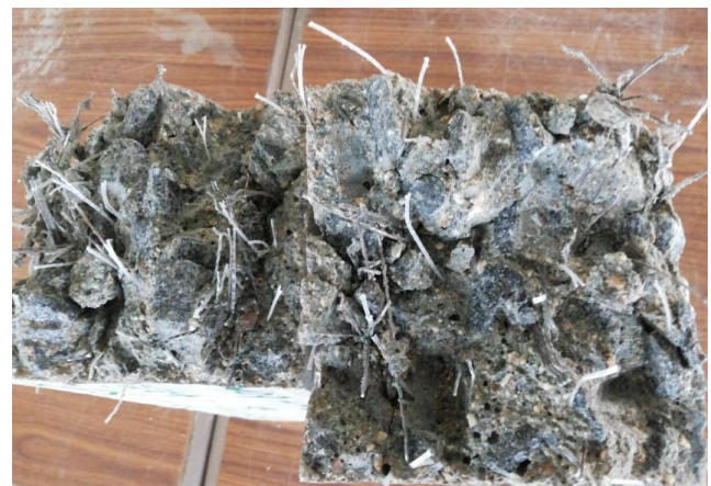
Fig. 7. Image of polypropylene effects on the concrete beam
