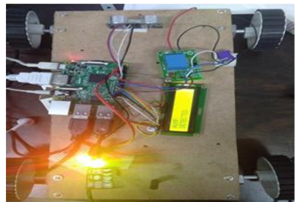
Fig. 20 LCD display when Hump is detected
