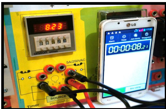
Figure 5. Timer on Delay Testing Source: personal document
