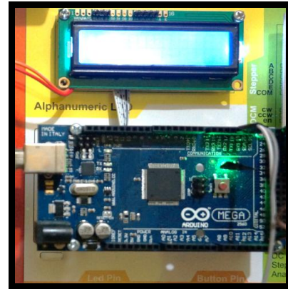
Figure 9. Modul RS 232 and LCD Testing Source: personal document
