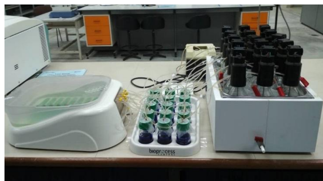
Fig. 3. Automatic Methane Potential Test System (AMPTS II) for BMP assay
