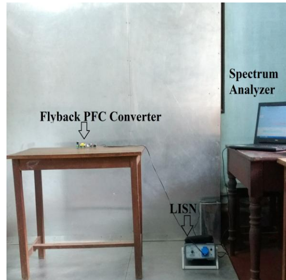
Fig. 15. Conducted EMI pre-compliance test setup
