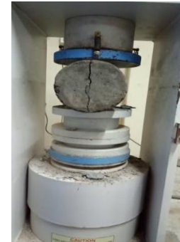
Fig: 10 Failure of cylinder
