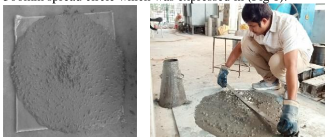
Fig: 1 Slump Flow and T 500 test
