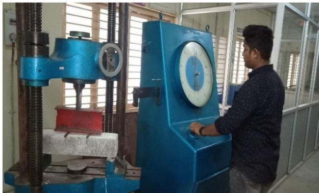
Fig: 12 Flexural Strength Test
