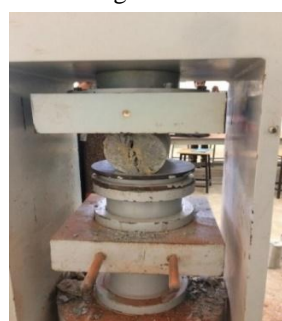
Fig.1 Experimental setup compression testing
