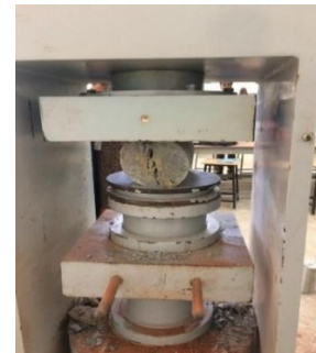
Fig.2 Experimental setup split tensile strength test
