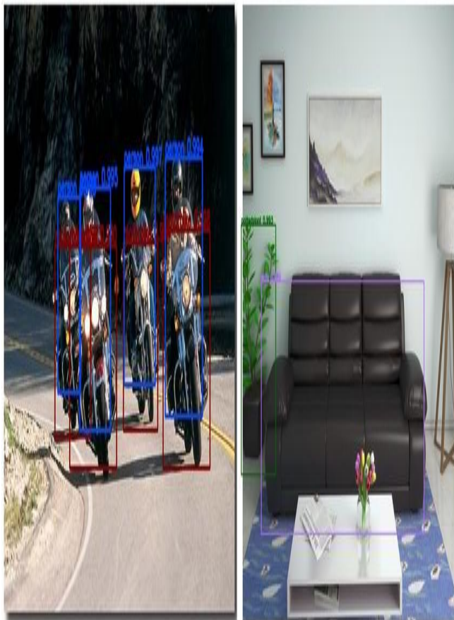
Fig. 8. The Faster R-CNN results on test data. The model classifies objects with probabilities. It also localizes objects by using bounding boxes.
