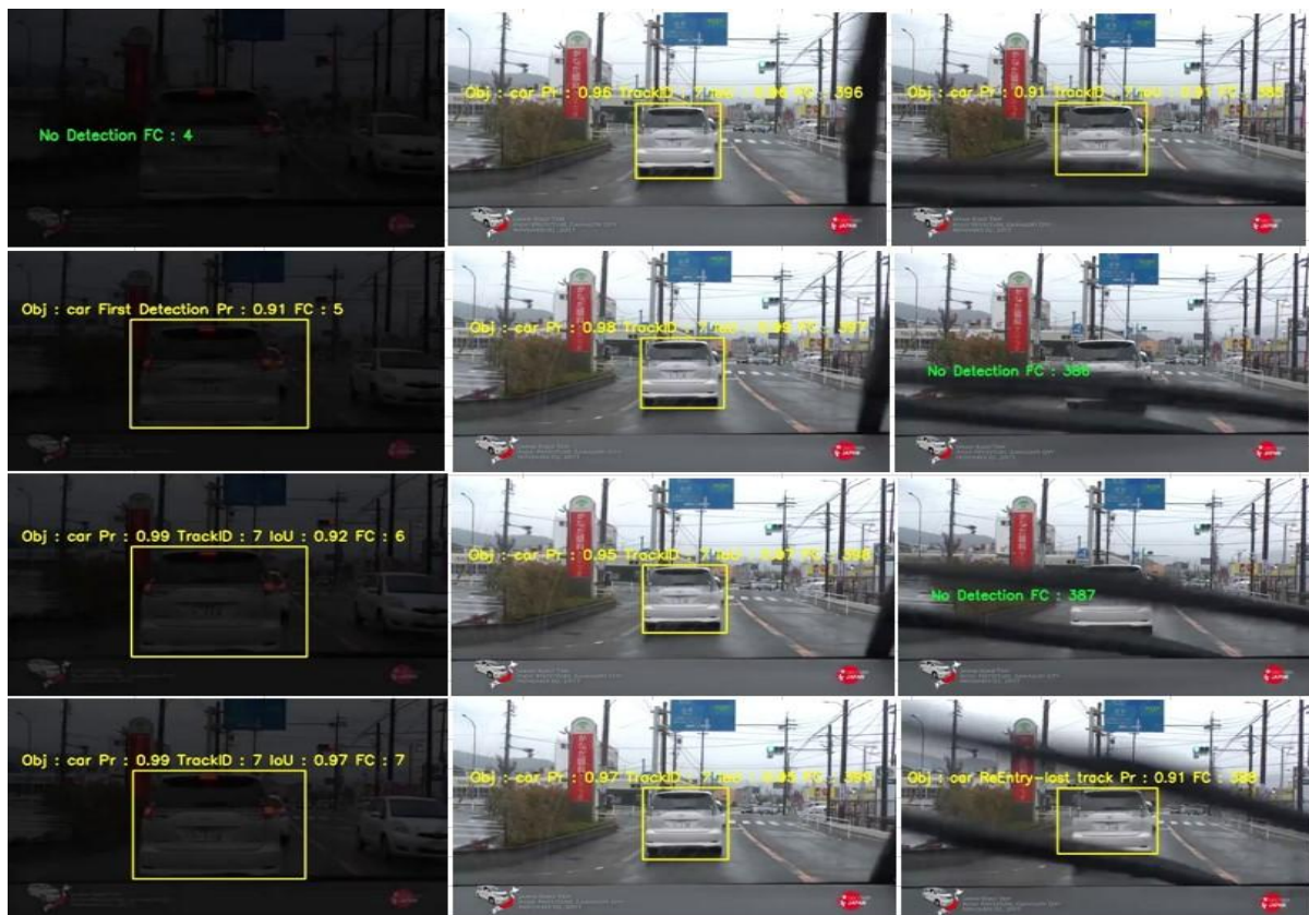
Fig.10. IoU tracking of object. In frame 4 (FC:4) there is no object detected. In frame 5 (FC:5), a new object car is detected which is then tracked in subsequent frames in FC:6, FC:7 and further. One unique tracking id is assigned to each class. IoU scores are also provided.
