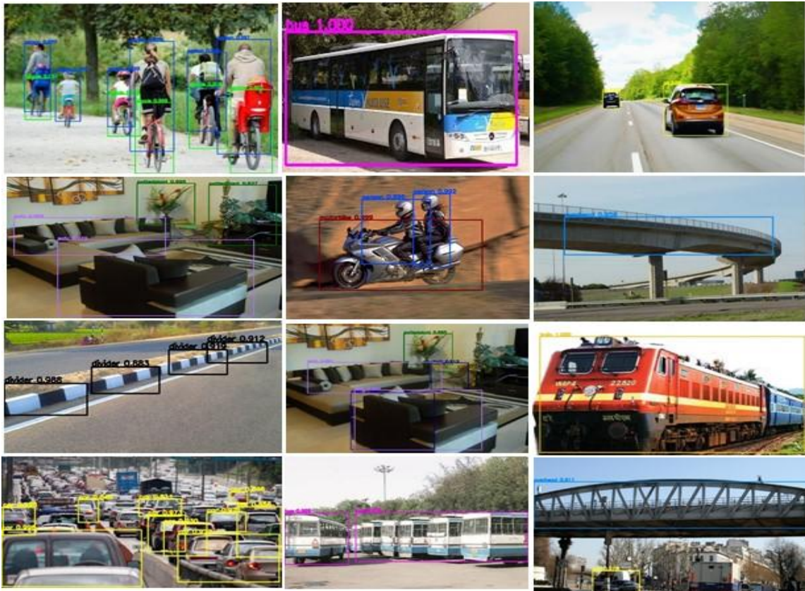
Fig. 9. More results of Faster R-CNN on test images using ResNet-101. Frames are processed at 5 fps.
