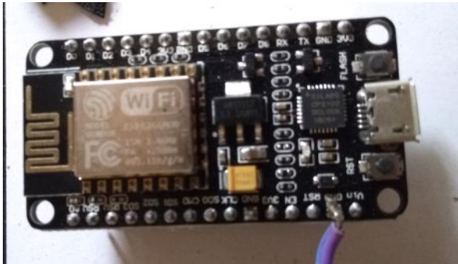
Figure 6: WiFi Module – ESP 8266.
