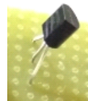
Figure 3: Temperature Sensor – LM35.
