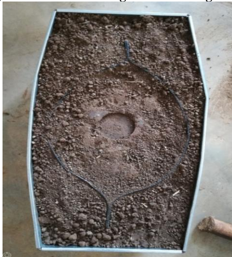
Fig.2. Modified CBR Mould with Subgrade & Geocell The analysis of pavement thickness is carried out by using KENPAVE software developed by Dr. Yang H, Huang, P.E., University of Kentucky.
