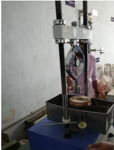
Fig.1. California Bearing Ratio Loading Frame
