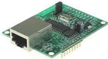
Fig.3.(c). Ethernet Board
