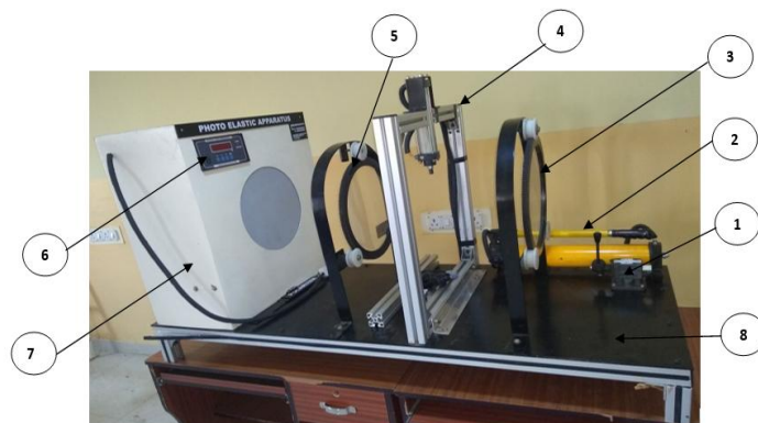
1. One directional valve, 2. Hydraulic pump, 3. Circular polariscope, 4. Mechanical load frame 5. Circular analyzer, 6. Digital load indicator, 7. Monochromatic light source, white light source 8. Leveling table
