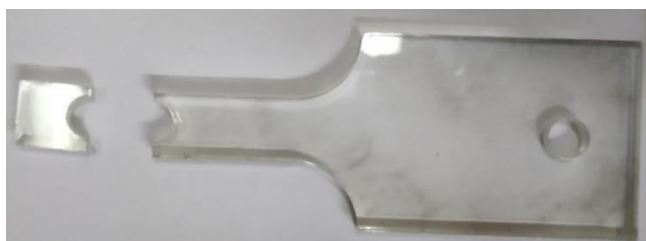
Fig. 18 Broken Sample of D/d = 3
