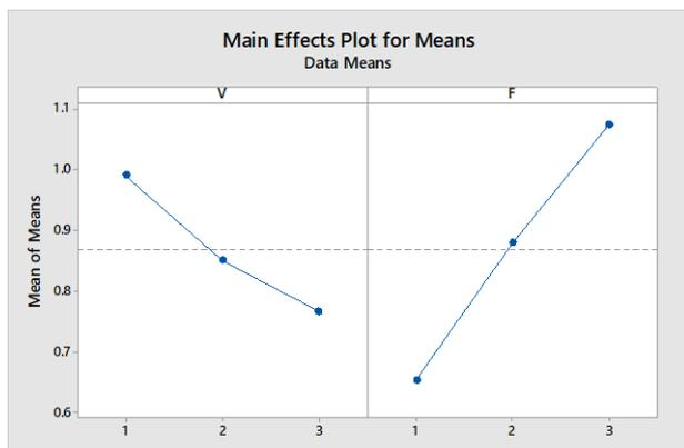
Fig. 3. Mean response table for  $R_a$ .
