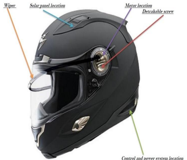
Figure 3. Solar panel and wiper installed in the system.
