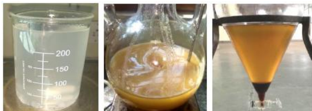
Figure 4: Methoxide, Transesterification process and Biofuel
