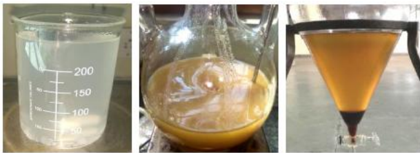
Figure 4: Methoxide, Transesterification process and Biofuel
