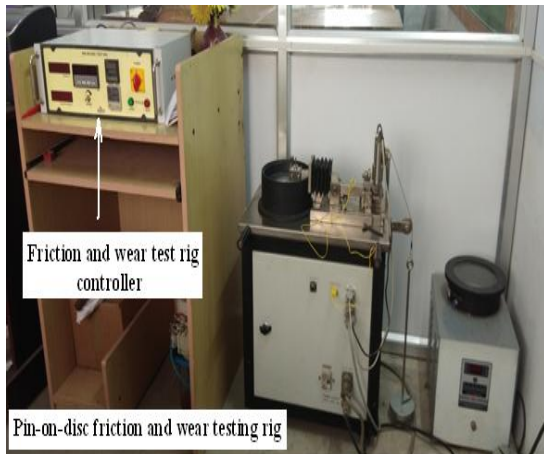
Figure 2: Schematic of pin-on-disc friction and wear testing rig
