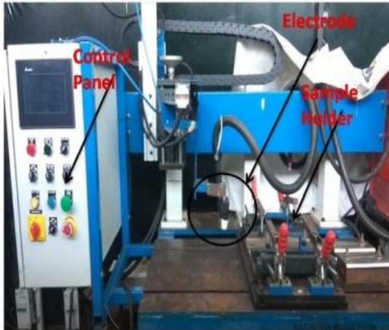
Fig.1 Schematic of TIG welding setup
