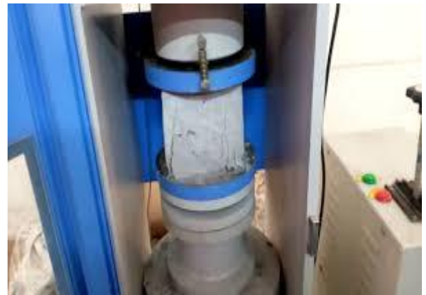
Fig: 4 compressive strength test of RO Waste water specimen
