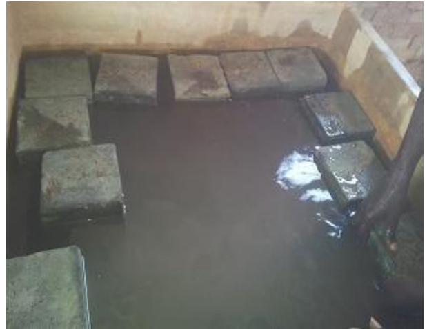
Fig: 3 curing of concrete specimen in RO waste water
