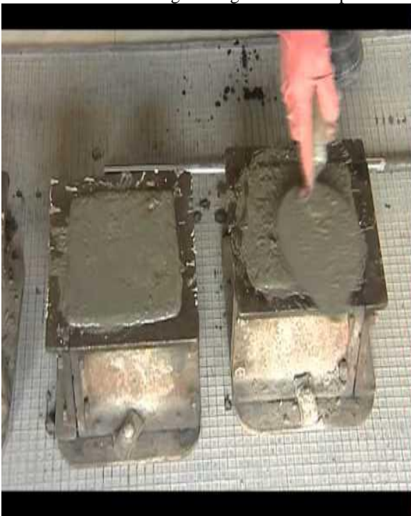
Fig: 2 casting of concrete cubes using RO waste water
