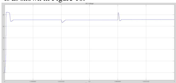
Figure 10 : DC output from three phase rectifier
