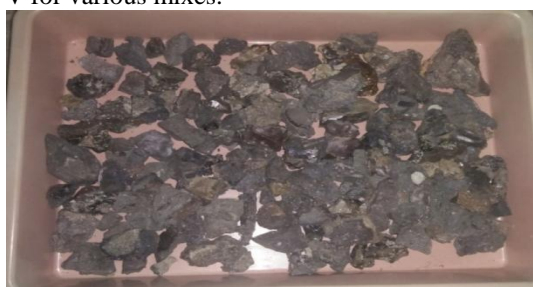
Fig. 1. Image of sintered metal steel slags
