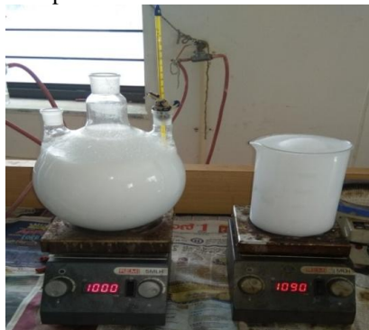
Fig. 3. Nanoparticles are mixed in a base fluid using a Magnetic stirrer
