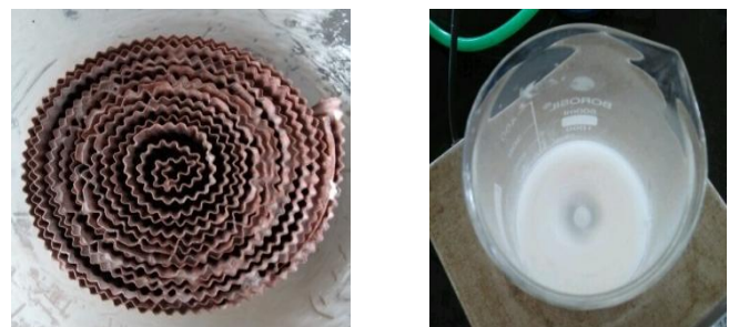
Fig.13 (a) prepared copper monolith, (b) mixture of metal catalyst and wash coat slurry
