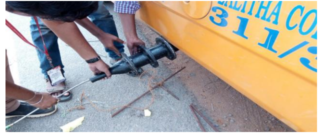
Fig. 16. On road vehicle Testing fitted with catalytic converter.
