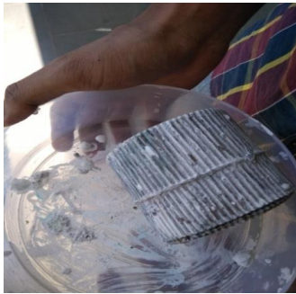
Fig. 15. Cerium oxide coated copper monolith substrate
