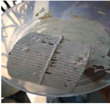
Fig. 14. ZrO 2 coated Copper monolith substrate
