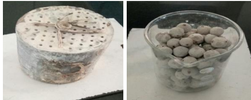
Fig. 8. Wash coat and catalyst coated SS Discs & Clay Marbles
