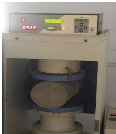
Fig. 3. Testing of Splitting Tensile Strength
