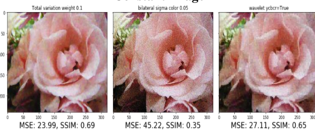
Fig v: (a) Fig v (b) Fig v(c) Fig: v (a)MSE&SSIM of Total variance Filter (case 1),v(b) MSE&SSIM of Bilateral Filter (case 1), v(c) MSE&SSIM of Wavelet denoising filter (case 1)
