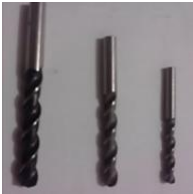
Fig 2. HSS and TAN coated carbide twist drill tool of tip angle of 118°
