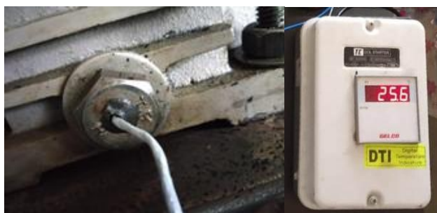
Fig. 2. Temperature sensor & its arrangement
