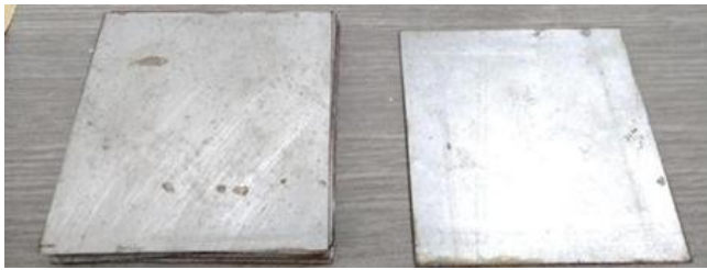
Fig. 2. 10x10 cm mild steel plate before cleaning (left) and after cleaning (right)
