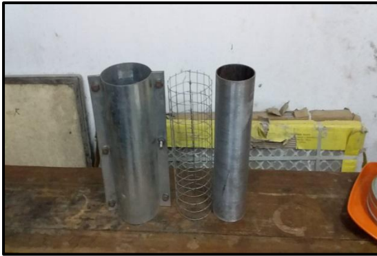
Fig no.2 cylindrical mould and reinforcement cage.
