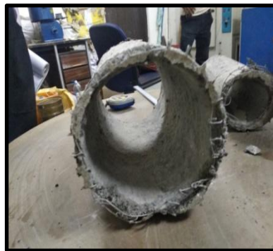
Fig no. 5(a), (b) & (c) showing failure pattern of the hollow reinforced concrete cylinders.
