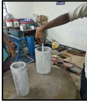
Fig no. 4(a), (b) Hollow concrete cylinders being measured
