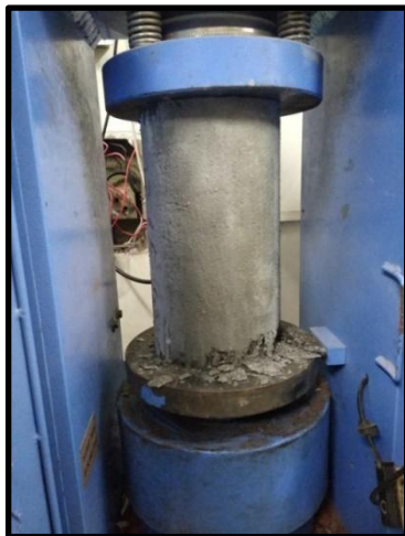
Fig no. 5(a), (b) & (c) showing failure pattern of the hollow reinforced concrete cylinders.
