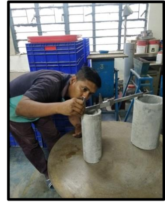
Fig no. 4(a), (b) Hollow concrete cylinders being measured
