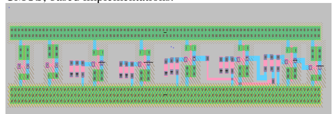
Fig. 9. Layout of resistive threshold based one bit magnitude comparator
