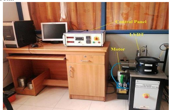
Fig. 1. Pin on Disc Tribometer Setup
