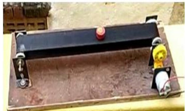
Fig.4. Mechanical assembly of conveyor 1
