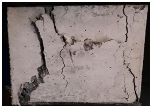
Fig. 7. Crack Pattern of Cube
