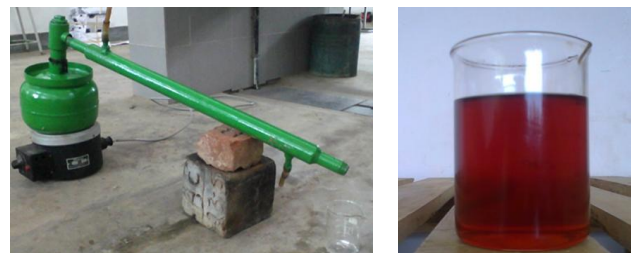
Figure 3. Solvent extraction and pupae oil
