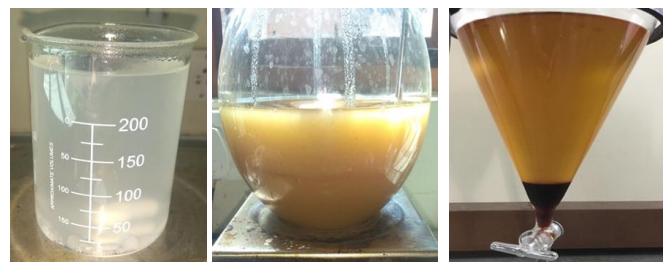
Figure 4. Methoxide, Transesterification process and Biofuel
