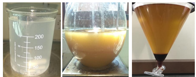
Figure 4. Methoxide, Transesterification process and Biofuel
