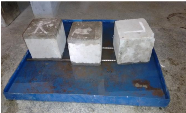
Fig 6 Sorptivity test on cube specimens
