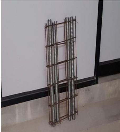
Fig 3. Precast wall – pipe sleeves
