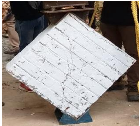
Fig.8 (c).PP geofabric Bed Joint Reinforcement
