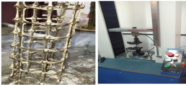
Fig.1. Polypropylene geo-fabric and testing arrangement in UTM
