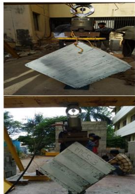
Fig.7. Diagonal Compression Test
