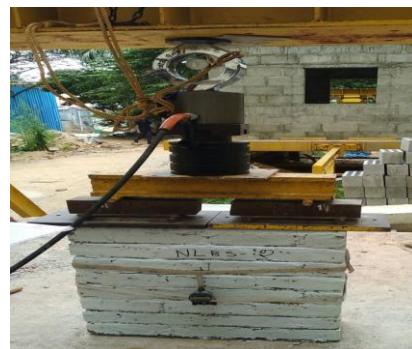
Fig.3. Load Bearing capacity test on Masonry wallet
