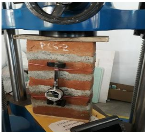
Fig.2. Compression test on masonry Prism
