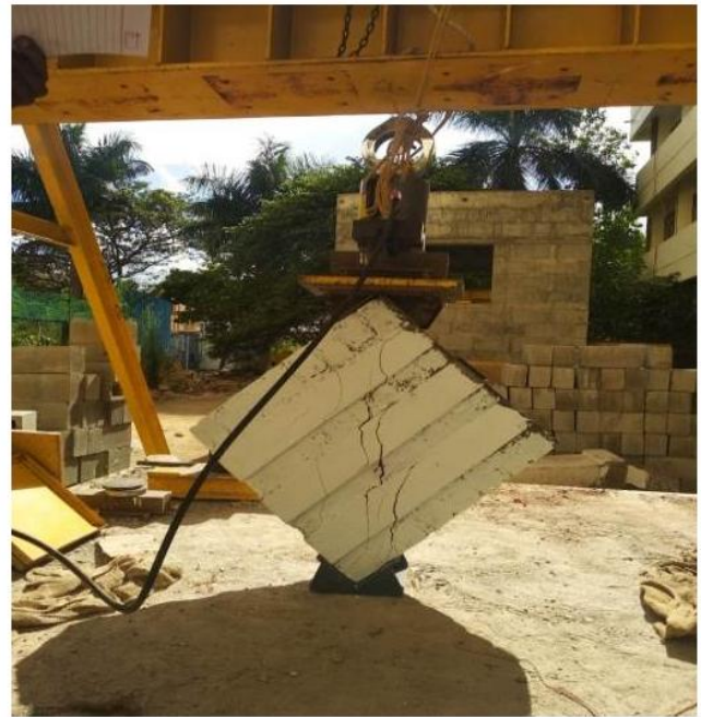
Fig.8 (b).PP geofabric face Reinforcement
