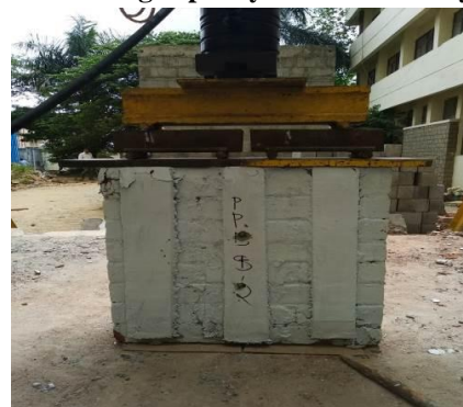
Fig.4. PP Geo-fabric Face strengthened wallet
