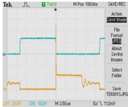
Figure 11: Measured voltages at MOSFET terminals for planar inductor circuit (CH1: V_{\text{drain-source}} , CH2: V_{\text{gate-source}} ).
